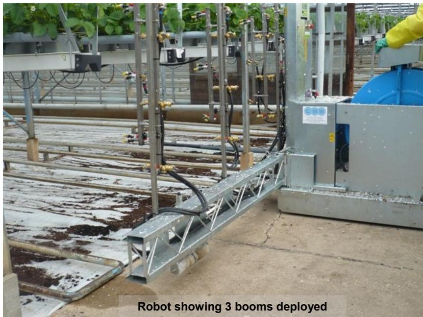
Robot showing 3 booms deployed
